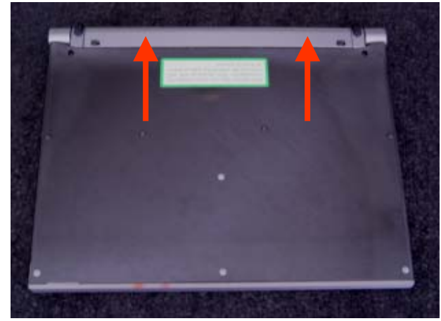
In the state 1), pull the Battery Pack in the arrow direction.
